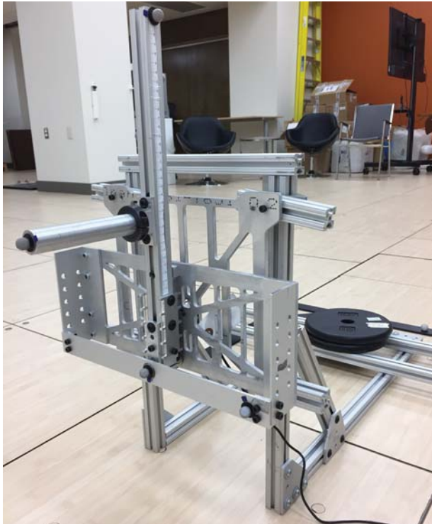
Figure 2: The device, without mass or springs, mounted to the testing apparatus.
